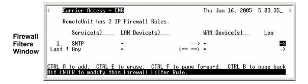
5. Enter the parameters of the rule, select [ESC] to close the window and save the configuration. See *page 5-30* for a description of all fields for the Firewall Setup window.
